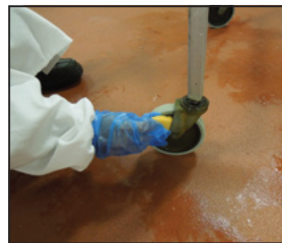
Equipment supports, floor anchors, and wheels are important swab-target sites. Swabbing deep into gaps and junctions is an important standard procedure to reduce the chance of missing a resident niche and biofilm build-up by Listeria
